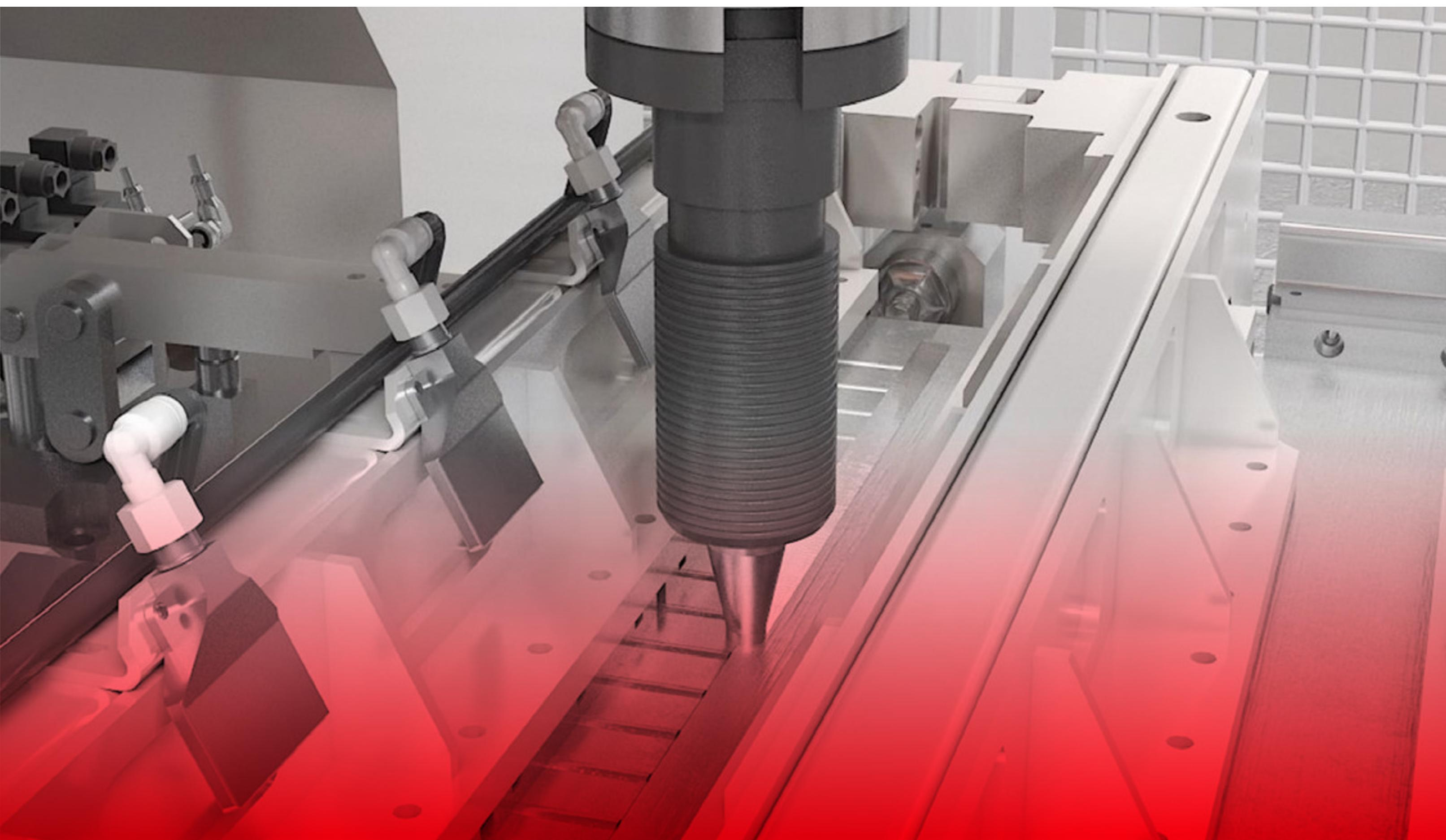
Friction stir welding (FSW) is a solid-state welding process that uses a non-consumable tool to join two materials by mechanical mixing without melting them, creating strong and reliable joints that can stand up to even the toughest operating conditions. This makes it an ideal process for battery trays.
