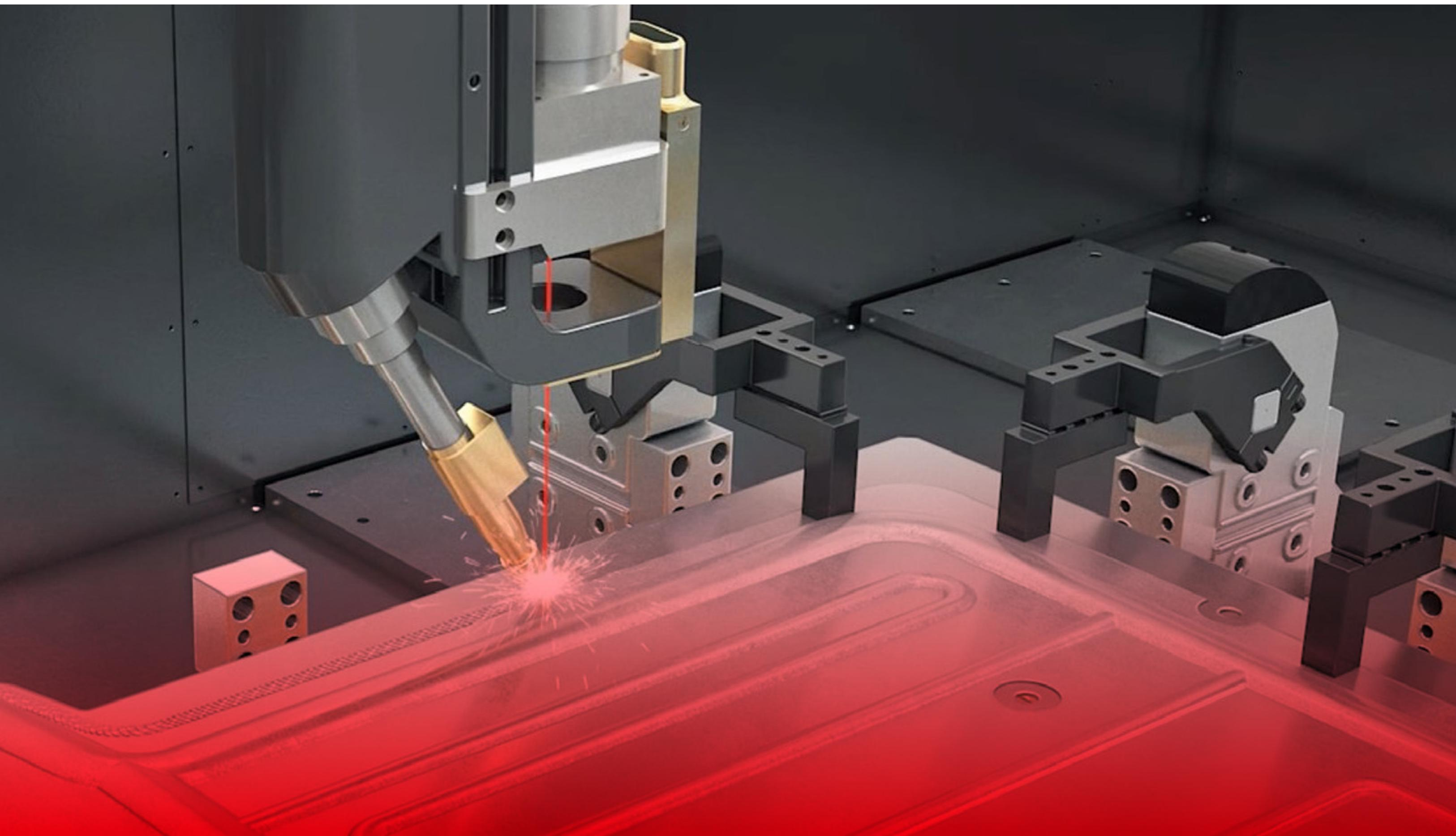
Laser welding provides a high-precision, high-speed solution for welding battery trays. This is essential for the automotive industry, which needs welds that are tough enough to withstand harsh operating conditions and have a narrow heat-affected zone.
